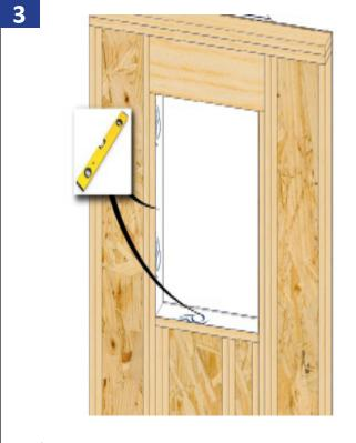
Verify the rough opening is plumb and level. The sill plate beneath the unit must be level for proper unit operation.
