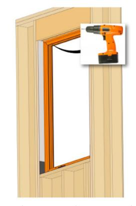
Temporarily fasten with a single fastener at the top of one jamb side as shown.
