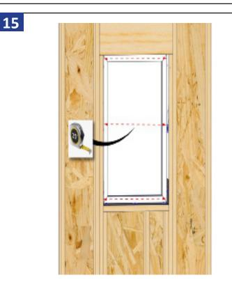
Check that the window is not bowed. Adjust shims as needed unit measurements are within 1/8".
