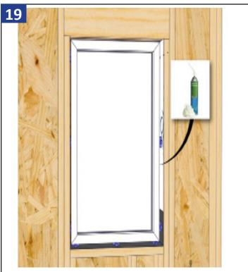
Fill interior 1/3 of the cavity using low expanding foam or loose insulation then seal the interior perimeter with silicone.
